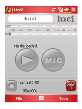
Start Luci Live two on both, choose the station (rtp int1 for the first in this example) and set them both to connect, like on the left. They will then both listen for an incoming stream on the RTP-port. As soon as one wants to talk, press on the Mic, the stream will arrive at the other end and the other listener hears the other talk and can decide to start talking also by pressing the Mic button.
